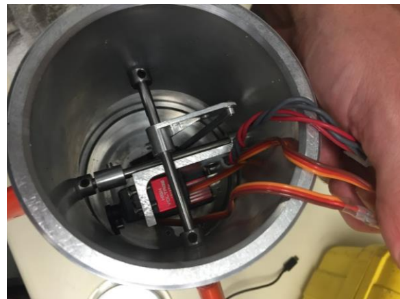
Figure 77: Servo Vessel Internals
