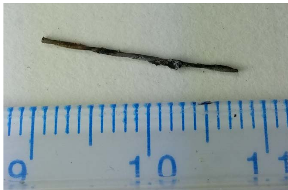
Figure 4.42 Forensic analysis of B1 SF2; cover depth 20mm Photograph by Dietrich Vogel copyright 2016 by Dietrich Vogel
