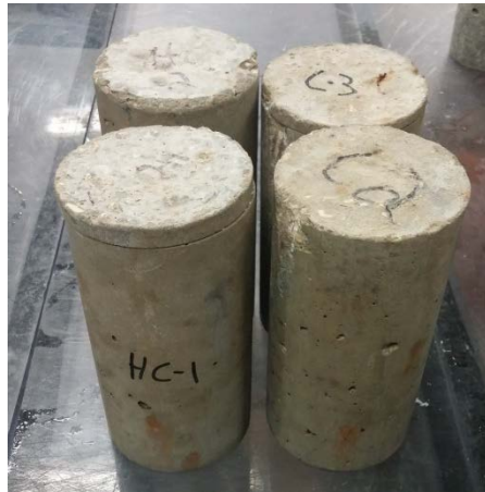
Figure 3.3 Non-instrumented samples cast with chlorides (HC1, HC2, C2, C3) Photograph by Dietrich Vogel copyright 2016 by Dietrich Vogel
