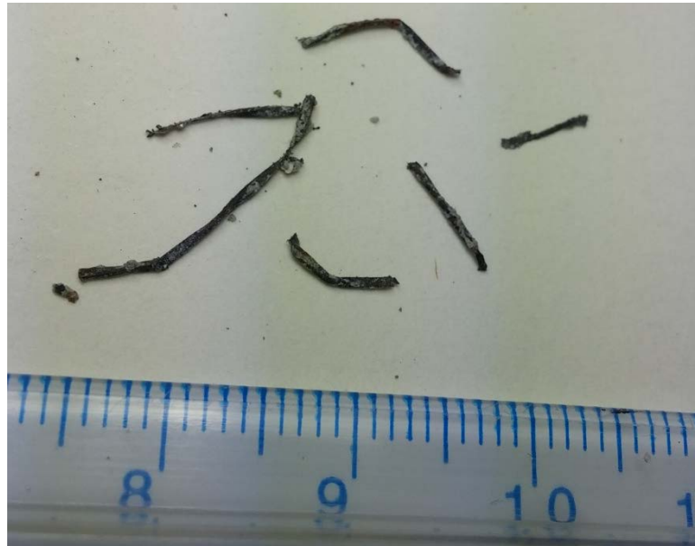
Figure 7.72 Slices approximately 2mm thick from RMT sample B after elevated temperature conditioning
