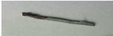
Figure 7.172 Carbon steel wires exposed on sample P2 8 months after casting
