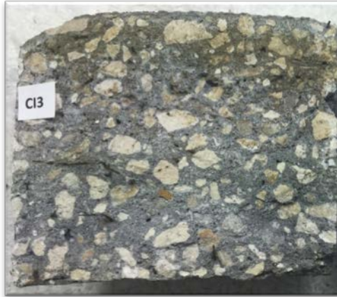
Figure 2.6 Sample CI3 sprayed with AgCl to indicate chloride migration Photograph by Dietrich Vogel copyright 2016 by Dietrich Vogel
