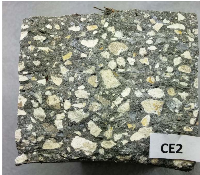
Figure 7.22 Beam CE2 post ASTM C78
