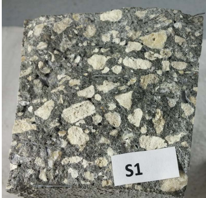
Figure 7.57 Failure plane 1 for beam S1
