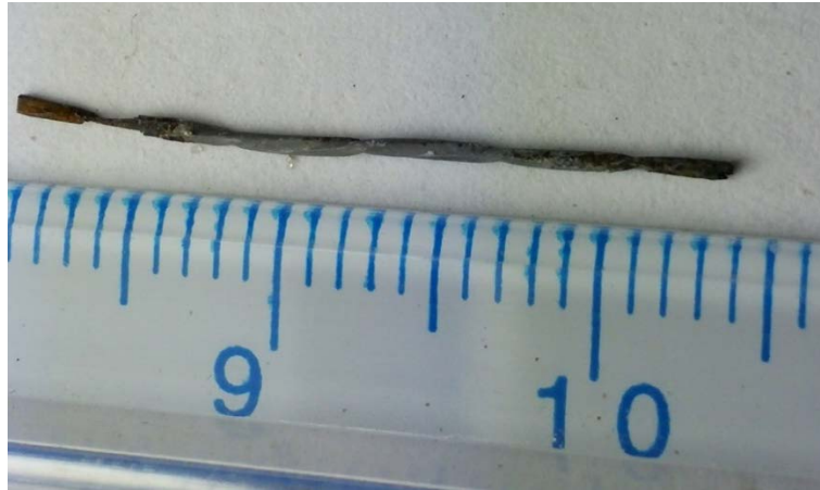
Figure 4.34 Forensic evaluation of MLWCA SF 13; cover depth 10mm Photograph by Dietrich Vogel copyright 2016 by Dietrich Vogel
