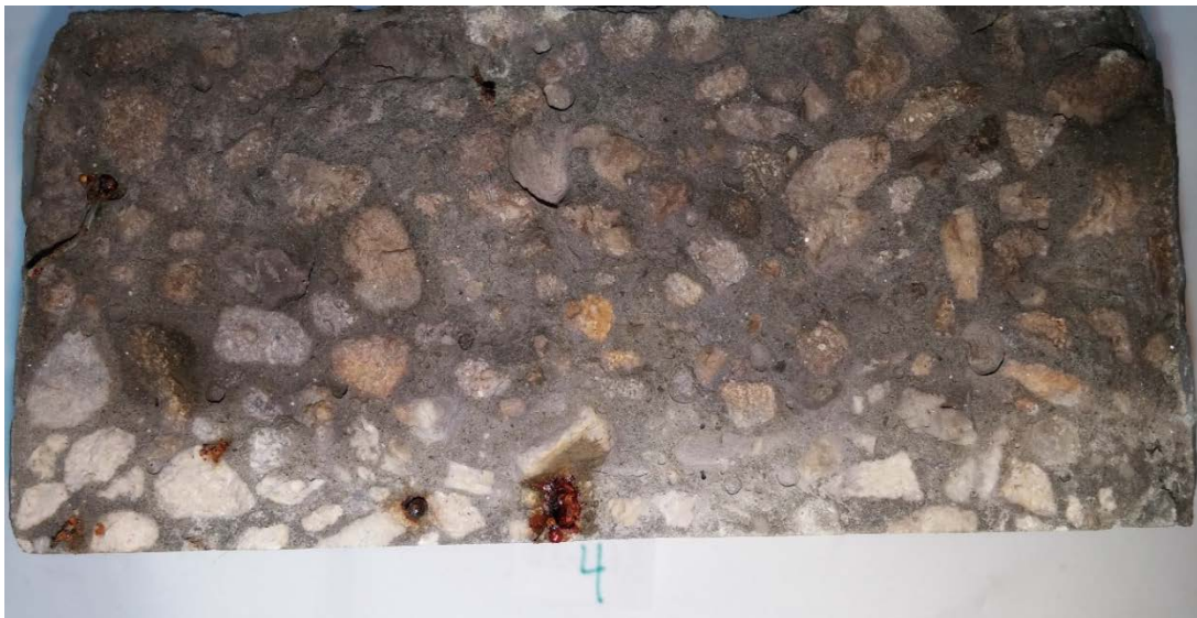
Figure 7.66 Slice 1 From NCB after being sprayed with silver nitrate
