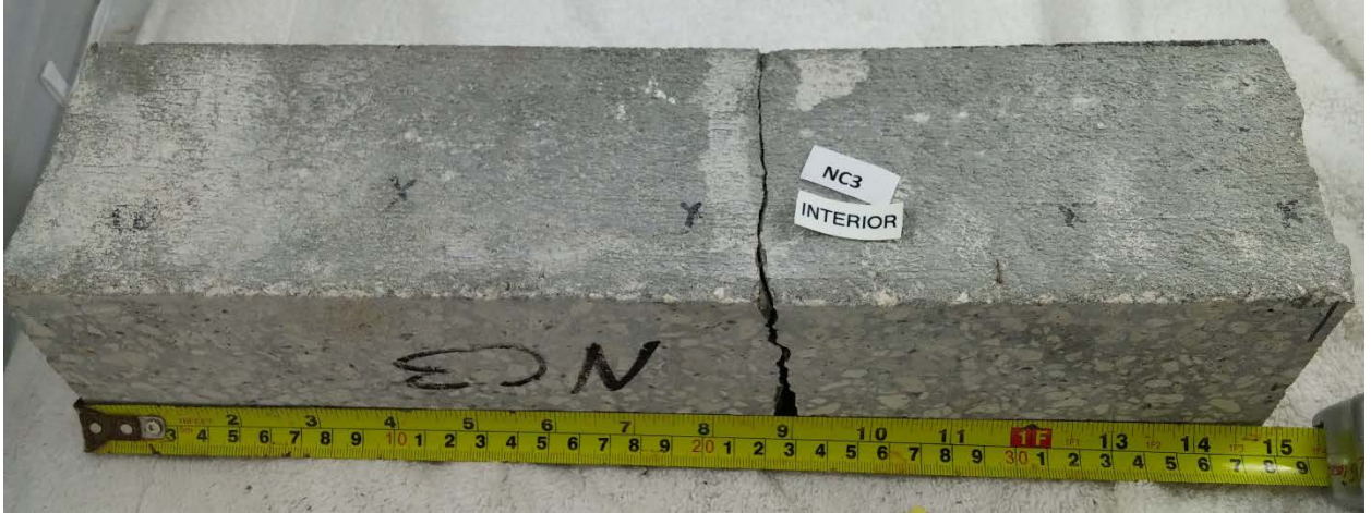
Figure 7.14 Beam NC3 post ASTM C78
