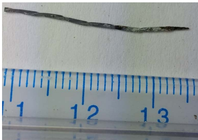
Figure 7.233 Carbon steel wire embedded in C8 without instrumentation
