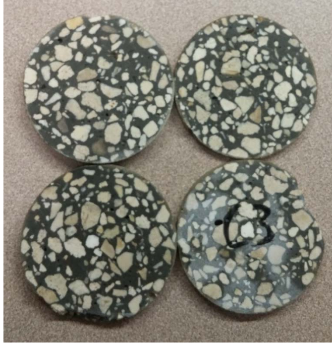
Figure 7.133 Four slices from cylinder C3 cut 6 months after casting with chlorides
