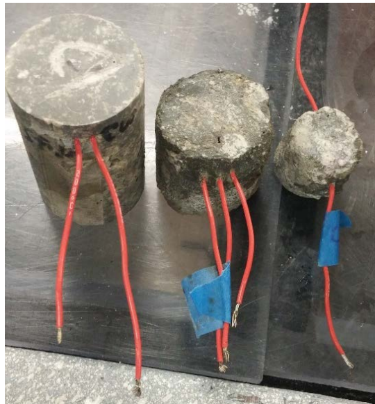
Figure 4.1 Instrumented Samples without chlorides(Left to right:C1, C5, C6) Photograph
