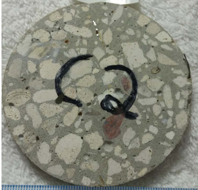
Figure 7.127 Slice C2 exposed to lab humidity for 5 weeks after cutting
