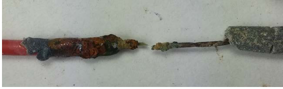
Figure 7.246 A3 fiber 1 coated in mortar
