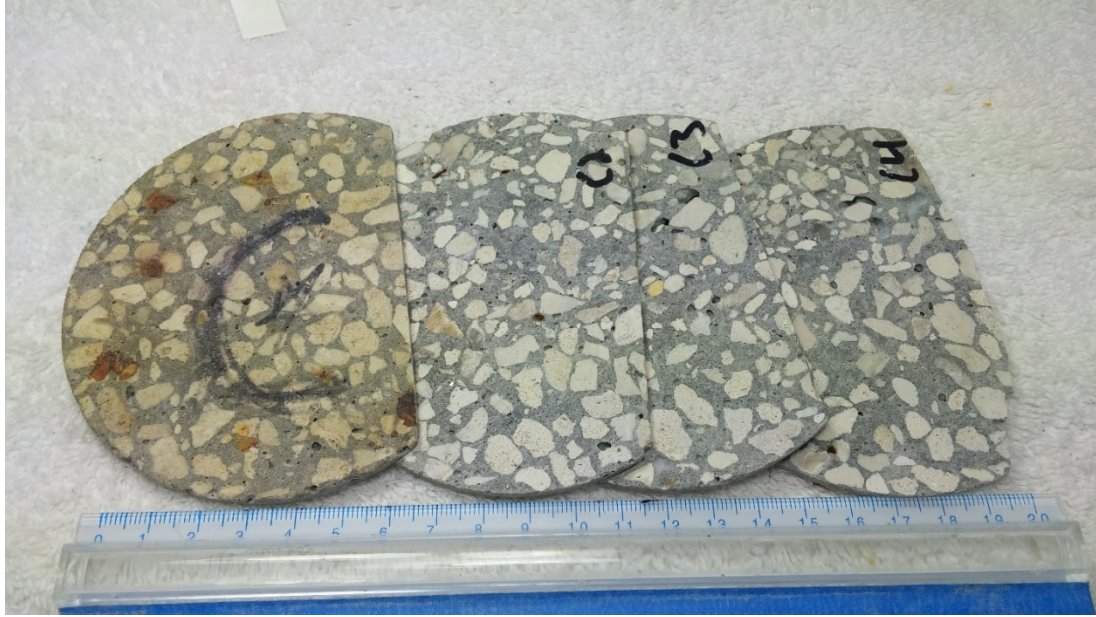
Figure 7.74 Slices approximately 2mm thick from RMT sample C after elevated temperature conditioning
