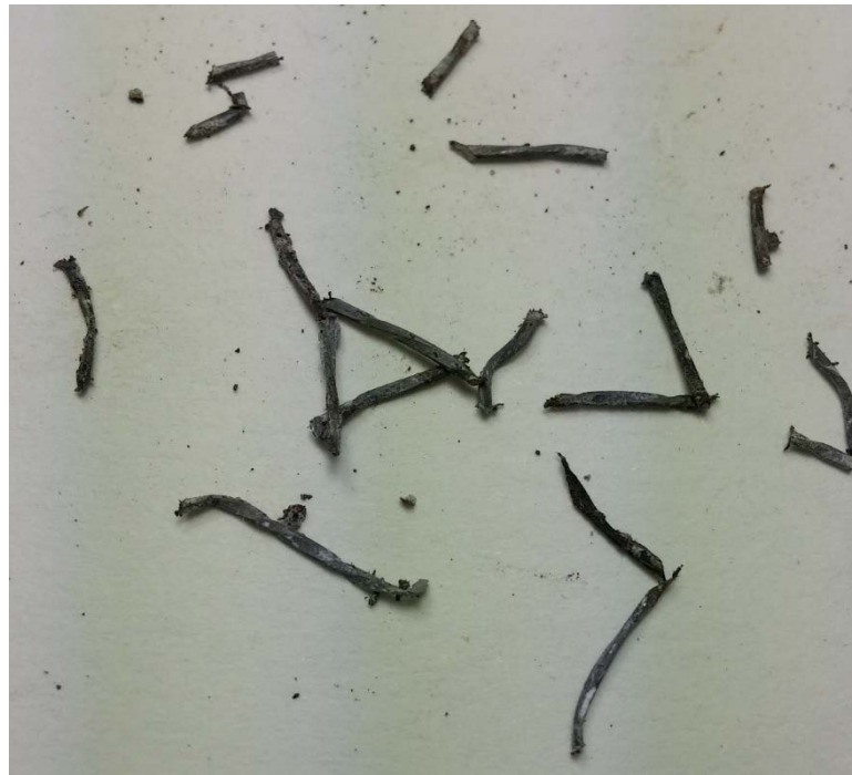
Figure 7.70 Slices approximately 2mm thick from RMT sample 3 after elevated temperature conditioning
