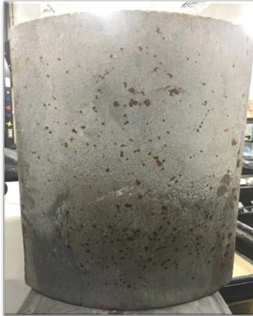
Figure 2.4 Pipe sample exposed to exterior chloride migration Photograph by Dietrich Vogel copyright 2016 by Dietrich Vogel
