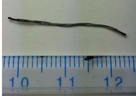
Figure 4.44 Forensic analysis of B1 SF4; cover depth 40mm Photograph by Dietrich Vogel copyright 2016 by Dietrich Vogel
