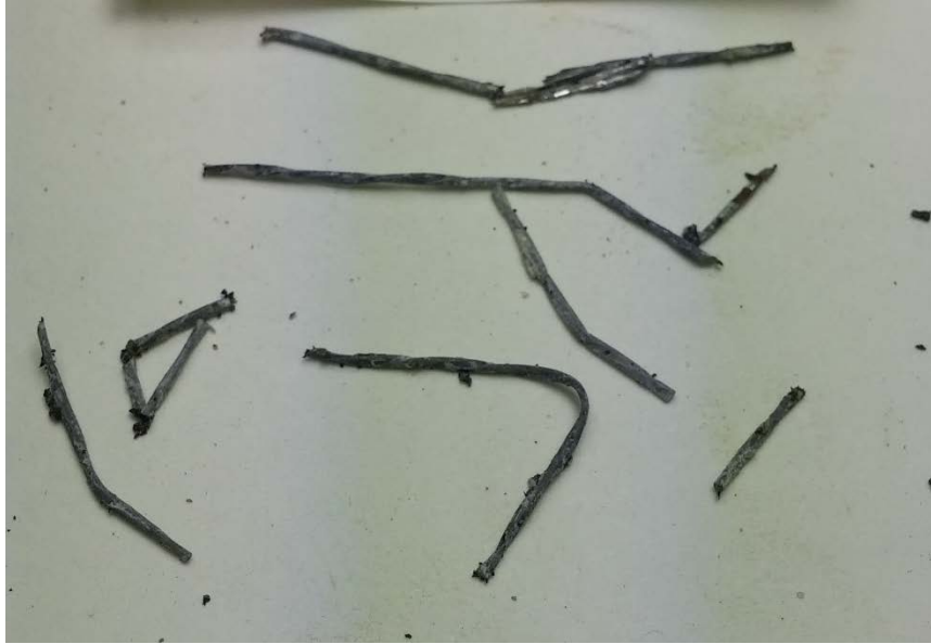
Figure 7.98 Fibers extracted from slice NCI exposed to high moisture and low oxygen
