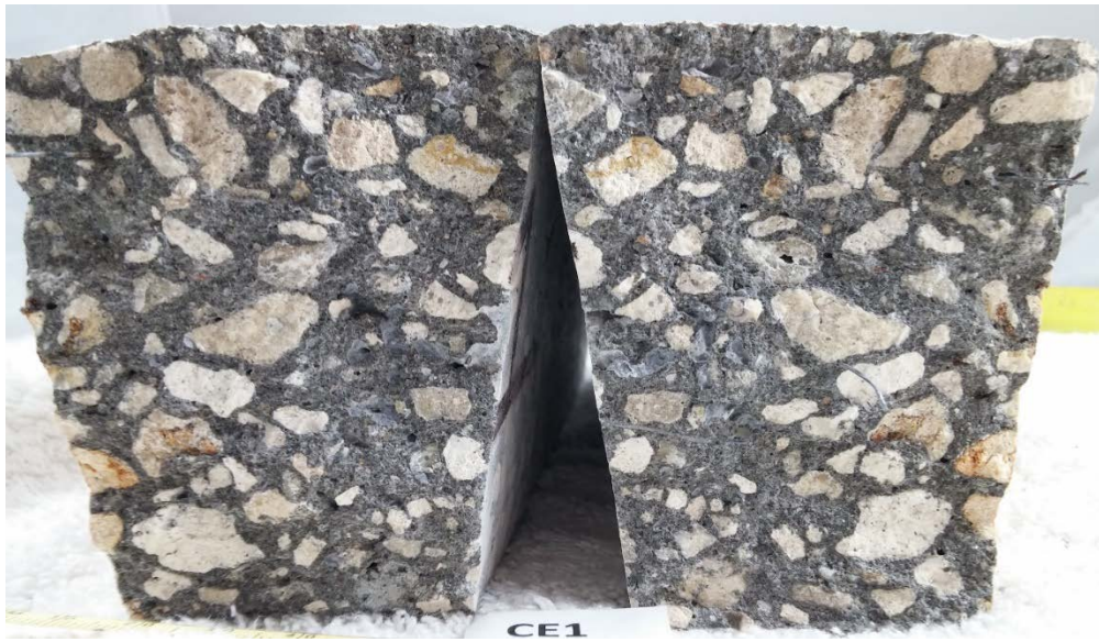
Figure 7.18 Beam CE1 post ASTM C78
