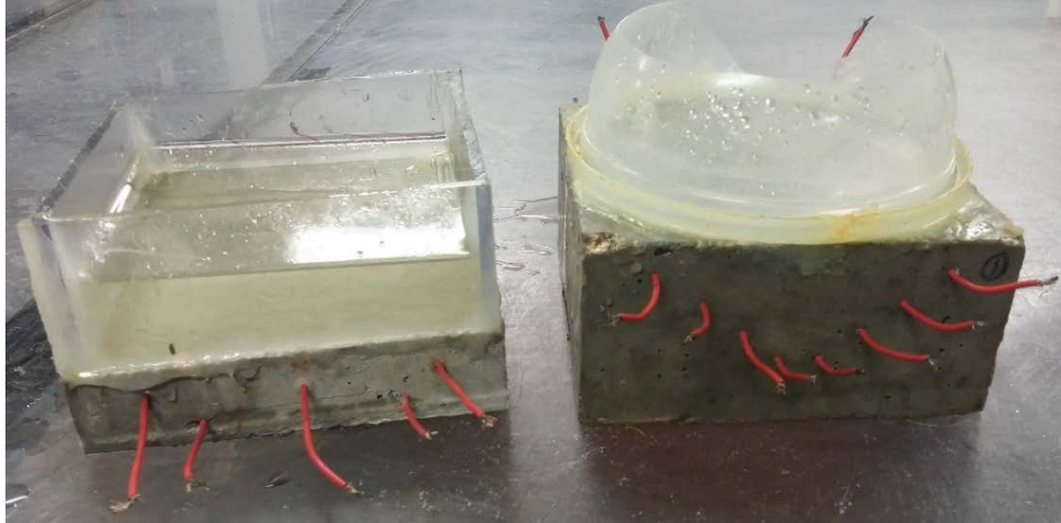
Figure 4.5 Migration block samples. (Left to right: B2, B1) Photograph by Dietrich Vogel
