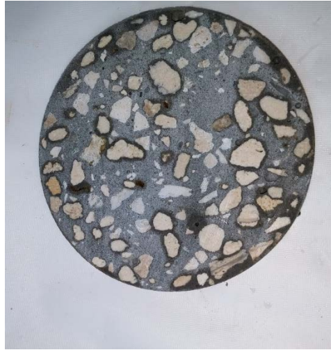
Figure 3.7 Sample NC after first slice taken 6 months after casting Photograph by Dietrich Vogel copyright 2016 by Dietrich Vogel
