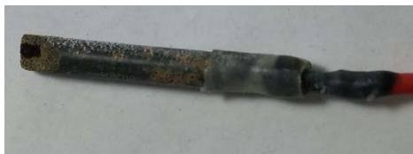
Figure 7.250 A3 fiber 3 coated in mortar post immersion
