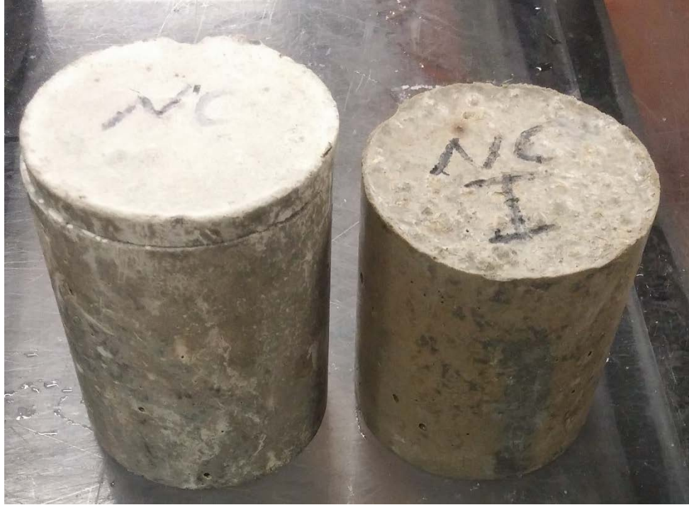
Figure 3.2 Non-instrumented samples cast without chlorides (NC, NCI) Photograph by Dietrich Vogel copyright 2016 by Dietrich Vogel
