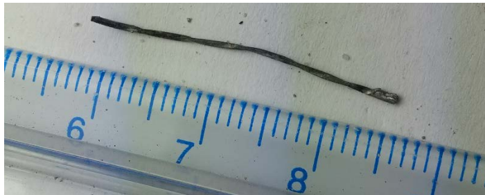
Figure 7.220 Instrumented SF3 at 10mm cover depth taken from sample B2
