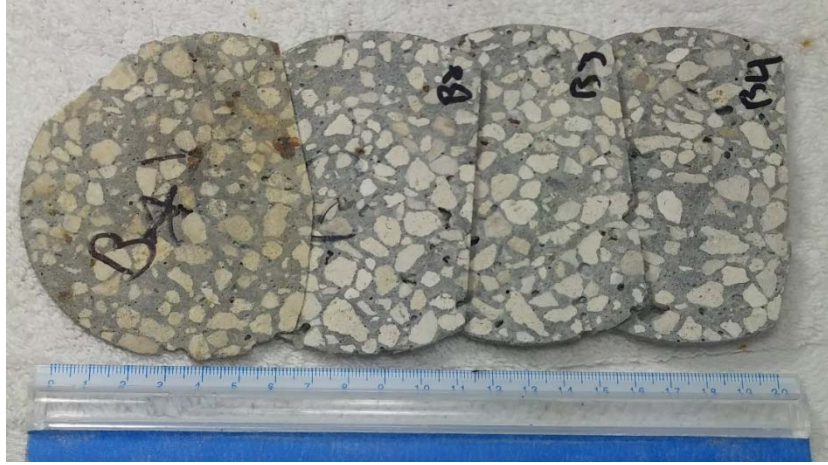
Figure 7.72 Slices approximately 2mm thick from RMT sample B after elevated temperature conditioning
