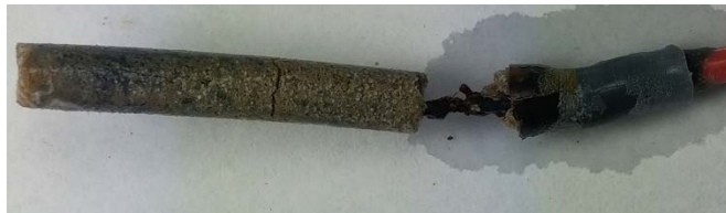
Figure 7.248 A3 fiber 2 coated in mortar post immersion
