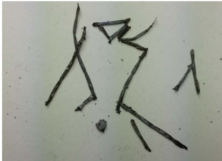
Figure 7.68 Slices approximately 2mm thick from RMT sample 2 after elevated temperature conditioning
