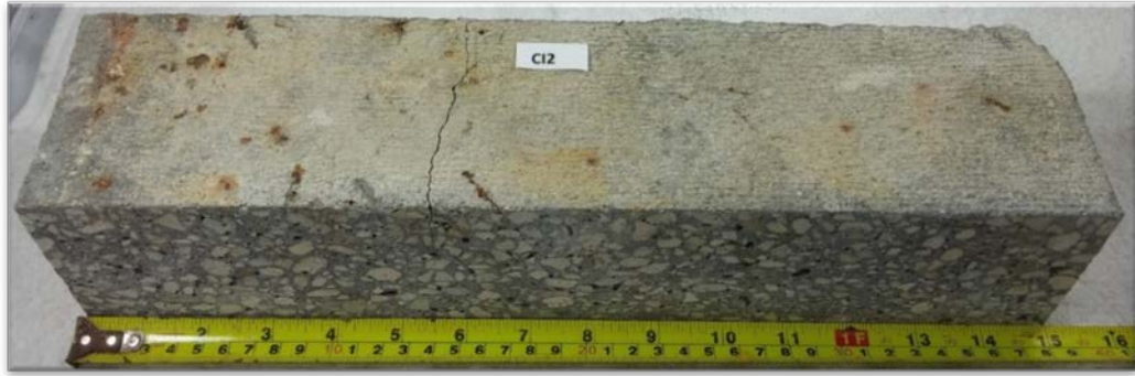
Figure 2.11 Beam sample CI2; modulus of rupture 805 PSI Photograph by Dietrich Vogel copyright 2016 by Dietrich Vogel
