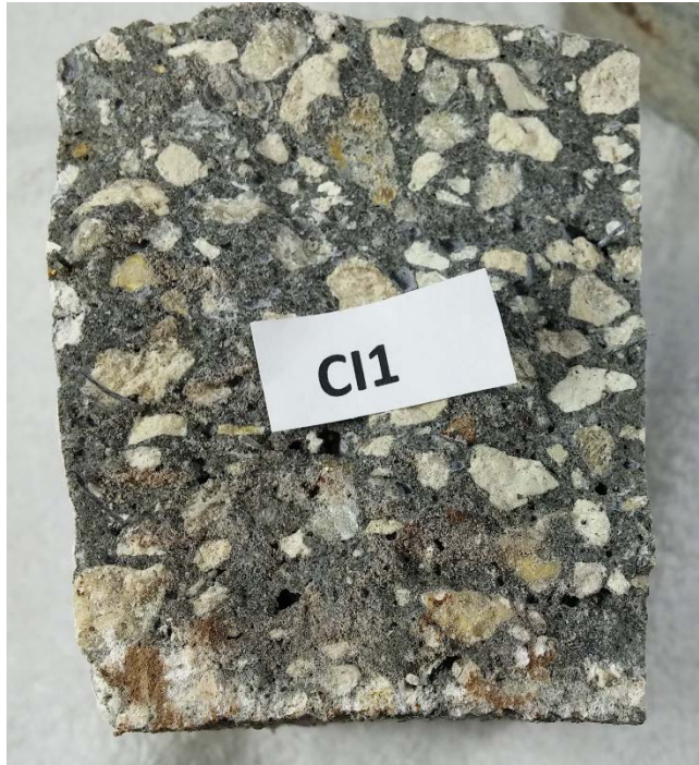
Figure 7.32 Beam CI1 post ASTM C78
