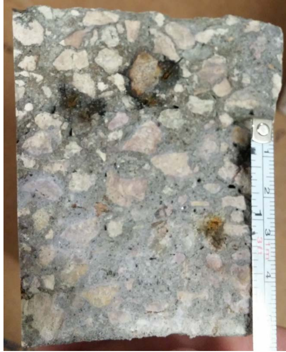
Figure 7.36 Failure plane from beam CI1 sprayed with silver nitrate
