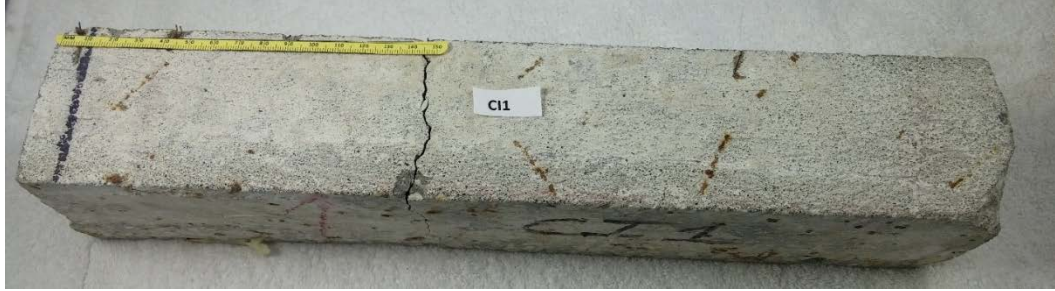
Figure 7.32 Beam CI1 post ASTM C78
