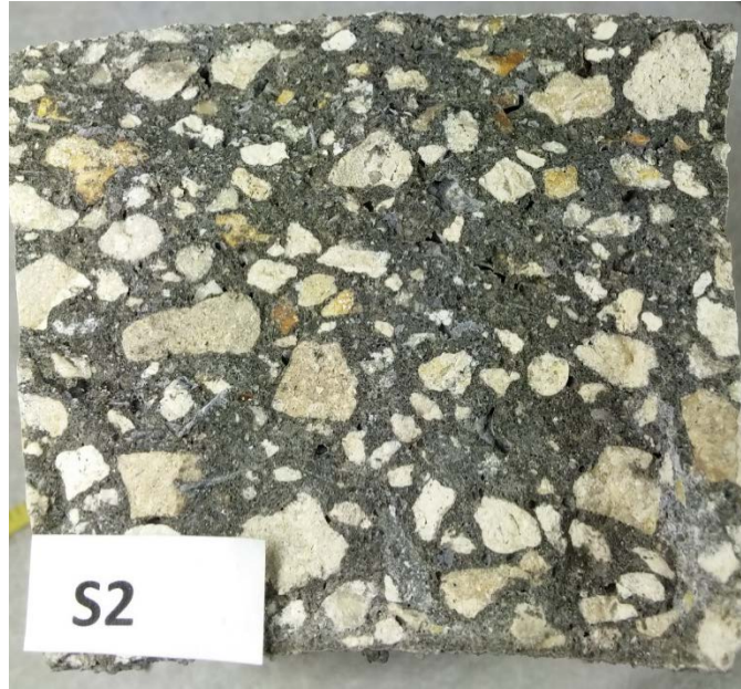
Figure 7.61 Failure plane 1 for beam S2
