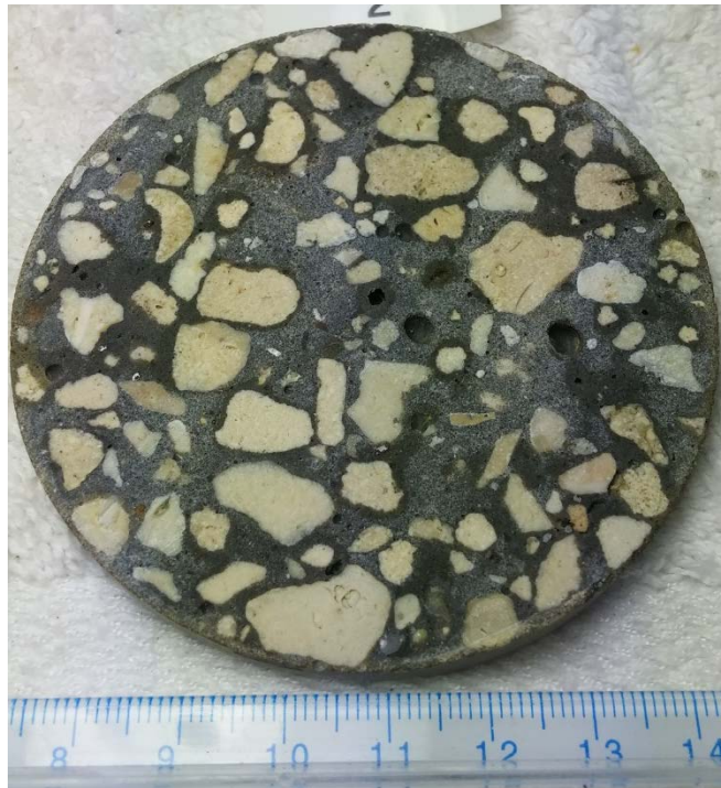
Figure 7.108 Slice HC1 after 5 weeks of high moisture and limited oxygen exposure
