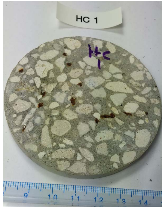
Figure 3.14 Disk sample HC1 after 5 weeks of outdoor exposure Photograph by Dietrich Vogel copyright 2016 by Dietrich Vogel
