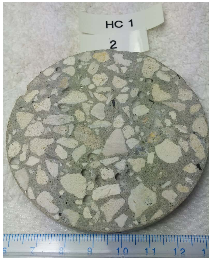
Figure 3.16 Disk HC1 exposed to inside conditions for 5 weeks Photograph by Dietrich Vogel copyright 2016 by Dietrich Vogel
