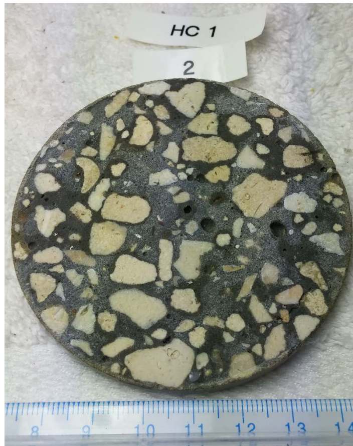
Figure 3.17 Disk HC1 Exposed to high humidity and restricted oxygen for 5 weeks Photograph by Dietrich Vogel copyright 2016 by Dietrich Vogel
