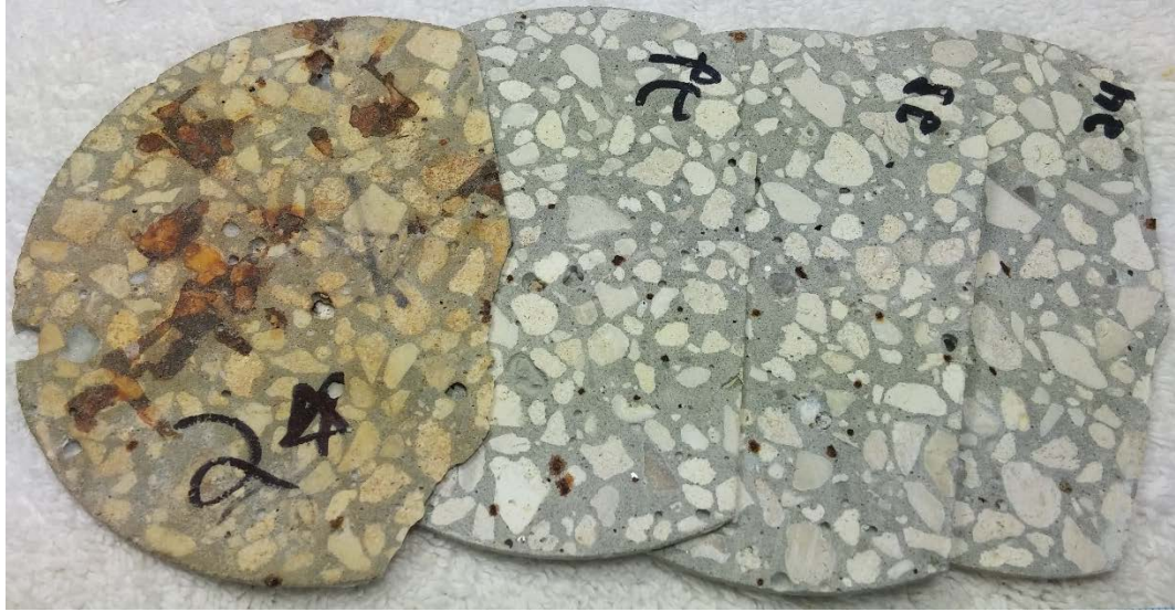
Figure 3.5 2mm slices taken from slice 2 of sample NCB after 4 weeks of lab humidity and oxygen exposure Photograph by Dietrich Vogel copyright 2016 by Dietrich Vogel
