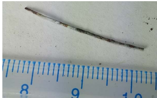
Figure 7.177 steel fibers while exposed from sample P2
