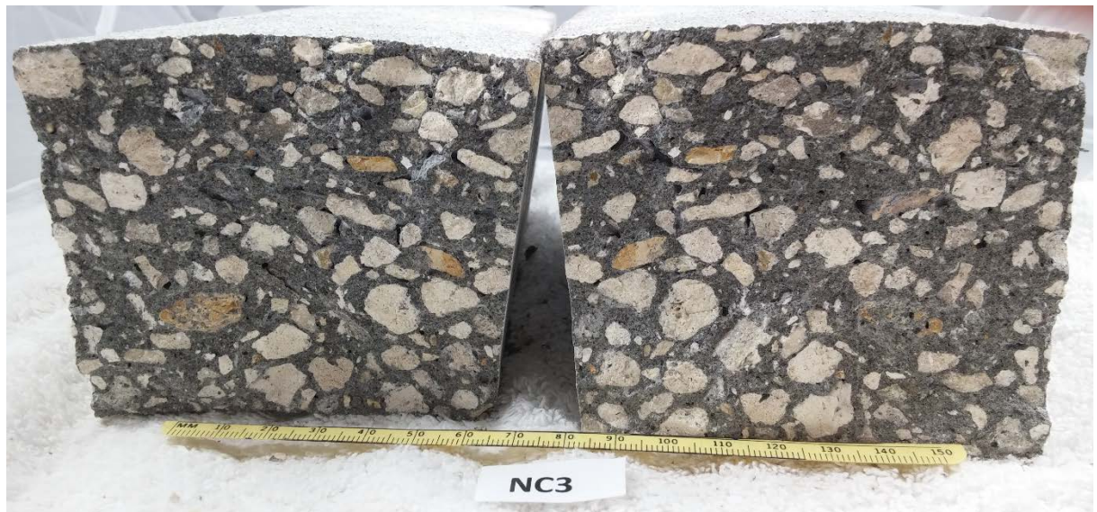
Figure 7.16 Failure plane 2 for beam NC3
