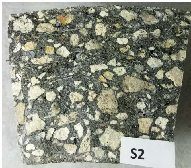
Figure 7.61 Failure plane 1 for beam S2
