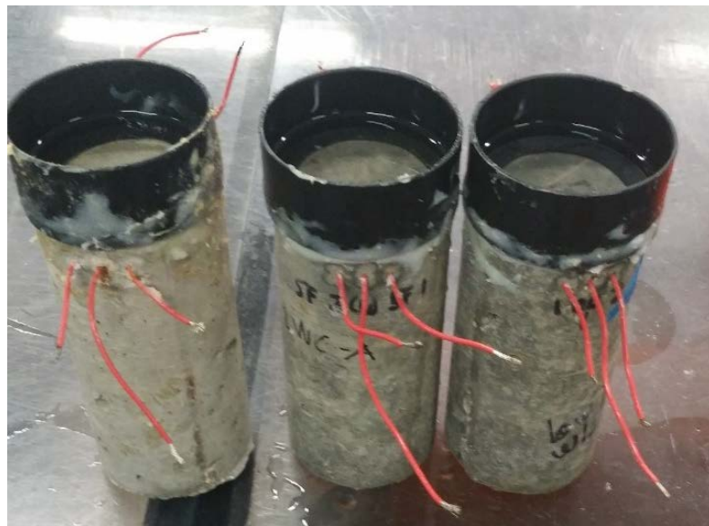
Figure 4.2 Instrumented samples cast without chlorides (Left to right: HWC, LWCA, LWCB) Photograph by Dietrich Vogel copyright 2016 by Dietrich Vogel
