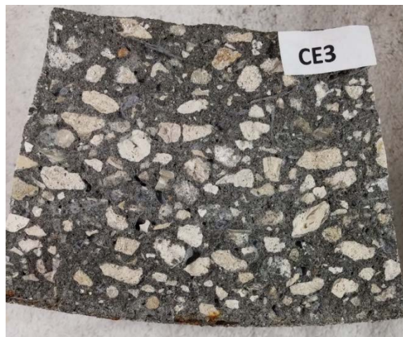
Figure 7.28 Failure plane 1 for beam CE3
