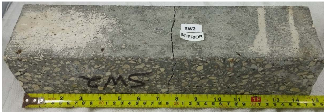
Figure 2.12 Beam sample SW2; modulus of rupture 895 PSI Photograph by Dietrich Vogel copyright 2016 by Dietrich Vogel
