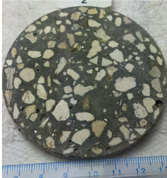
Figure 7.94 Slice NC exposed to high moisture and low oxygen for 5 weeks after cutting side 2
