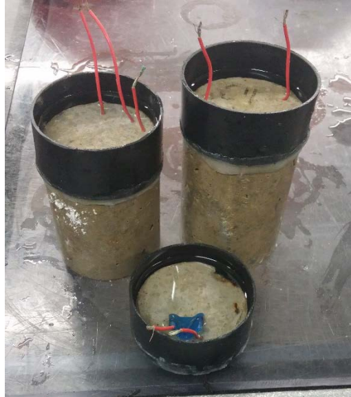
Figure 4.6 Instrumented sample cast with chlorides(Left-C8, Center-C7, Right-C4)
