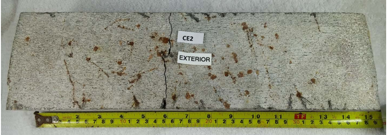
Figure 7.22 Beam CE2 post ASTM C78
