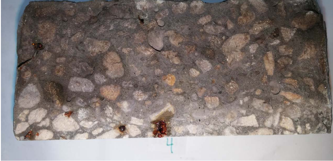
Figure 3.4 Core 4 from NCB after RMT picture taken months after being split
