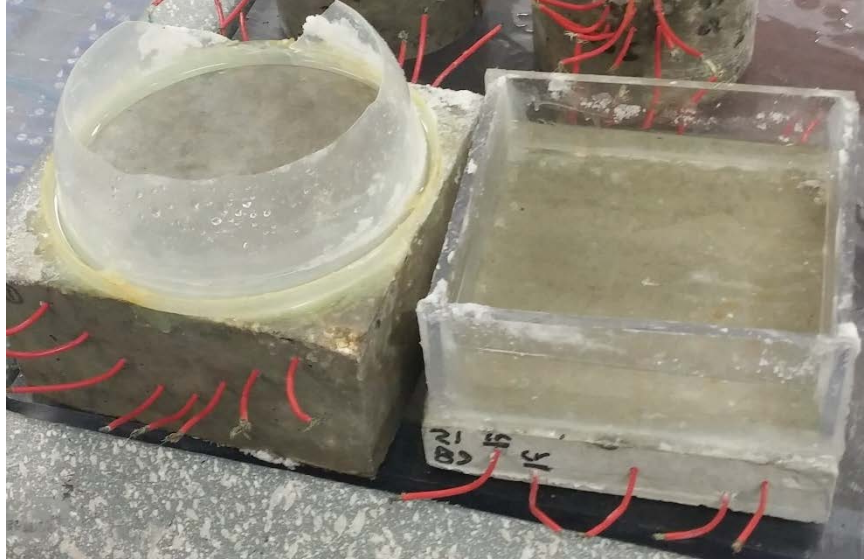
Figure 7.201 Sample B1 left and sample B2 right shown with reservoir ponds
