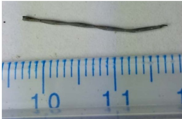
Figure 4.36 Forensic analysis of MLWCB SF 31; cover depth 30mm Photograph by Dietrich Vogel copyright 2016 by Dietrich Vogel
