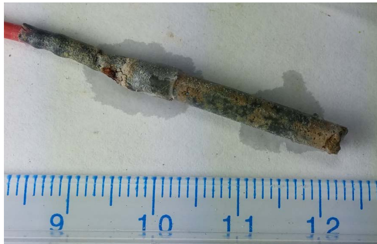
Figure 7.254 Carbon steel wire coated in mortar; A3 fiber 5
