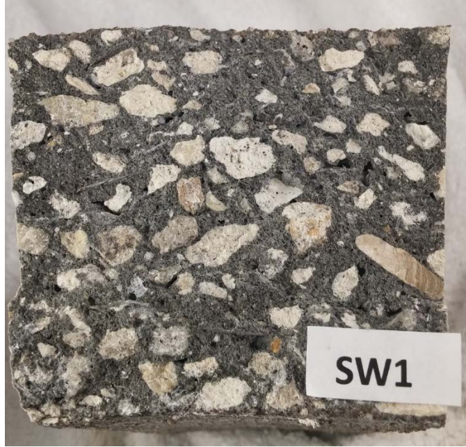
Figure 7.49 Failure plane 1 for beam SW1
