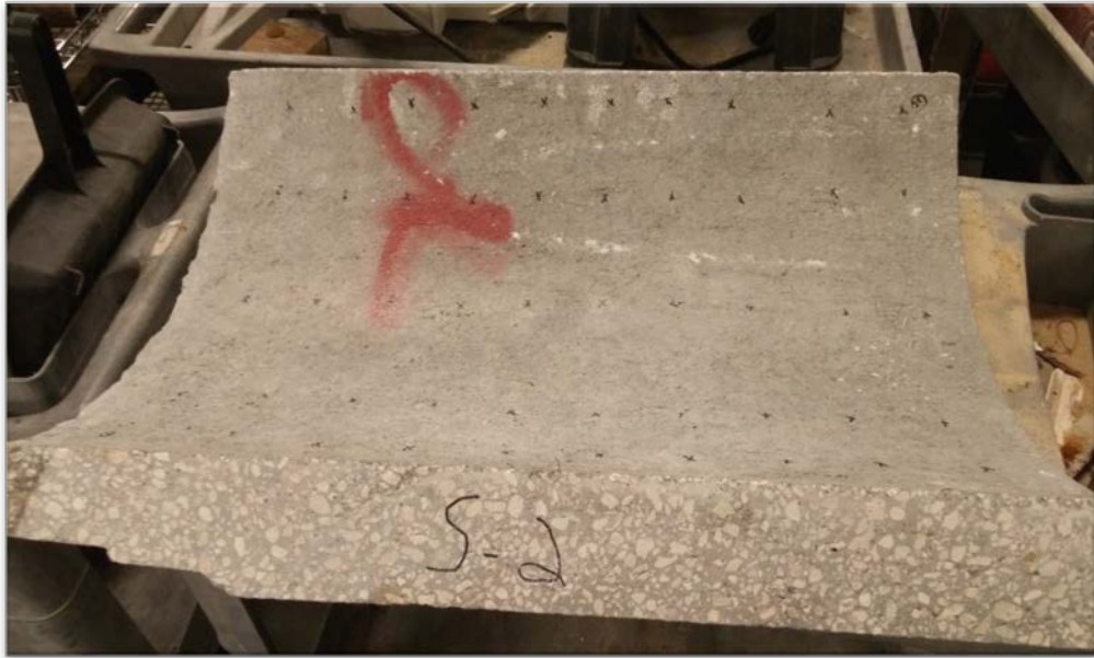
Figure 2.2 Pipe section S-2 made to be the no chloride control sample for beam bending Photograph by Dietrich Vogel copyright 2016 by Dietrich Vogel
