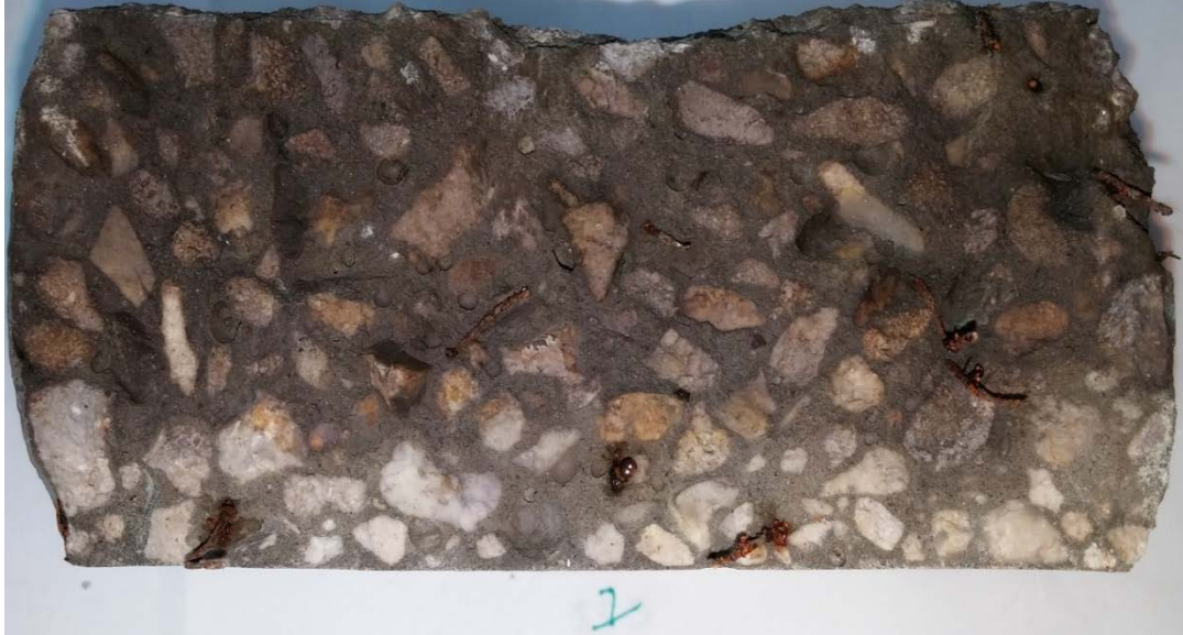
Figure 7.66 Slice 1 From NCB after being sprayed with silver nitrate
