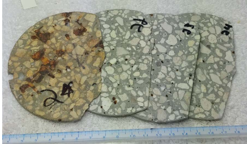
Figure 7.68 Slices approximately 2mm thick from RMT sample 2 after elevated temperature conditioning
