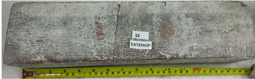
Figure 2.13 Beam Sample S2; modulus of rupture 940 PSI Photograph by Dietrich Vogel copyright 2016 by Dietrich Vogel
