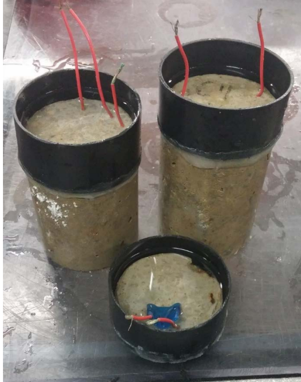
Figure 7.222 Samples cast with chlorides C8 left, C7 center, and C4 right
