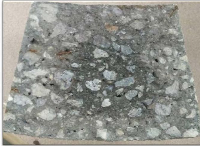
Figure 2.8 Sample SW2 after being sprayed with silver nitrate Photograph by Dietrich Vogel copyright 2016 by Dietrich Vogel
