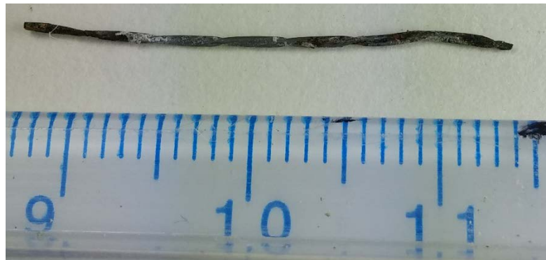
Figure 4.43 Forensic analysis of B1 SF3; cover depth 30mm Photograph by Dietrich Vogel copyright 2016 by Dietrich Vogel
