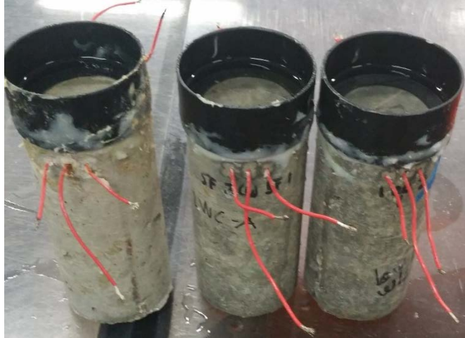
Figure 7.152 Cylinders subject to passive chloride migration HWC right, LWCA center and LWCB right
