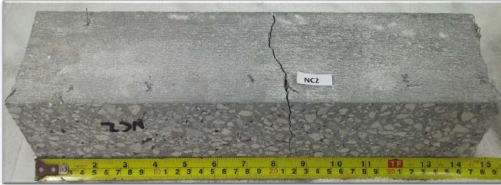
Figure 2.9 Beam NC2; modulus of rupture 1030 PSI Photograph by Dietrich Vogel copyright 2016 by Dietrich Vogel
