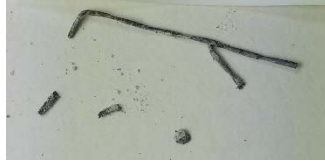
Figure 7.118 Fibers extracted from the HC2 slice left in lab humidity
