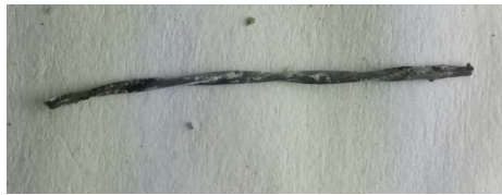
Figure 4.45 Forensic analysis of B2 SF 3; cover depth 12.5mm Photograph by Dietrich Vogel copyright 2016 by Dietrich Vogel
