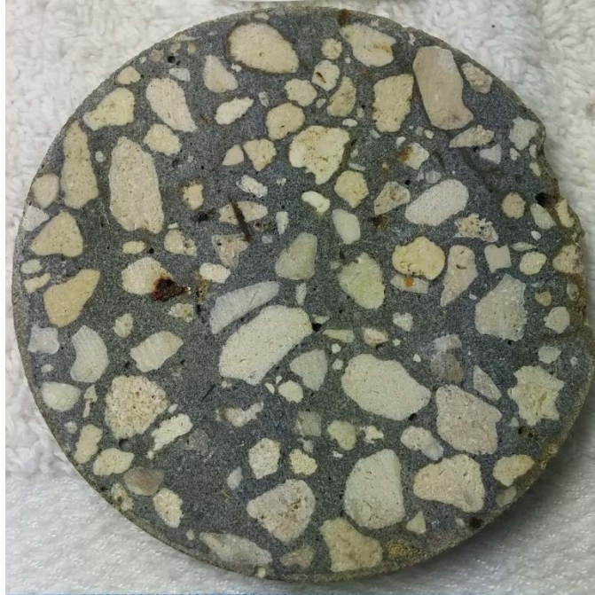
Figure 7.131 Slice C2 exposed to high moisture and low oxygen for 5 weeks after cutting side 2
